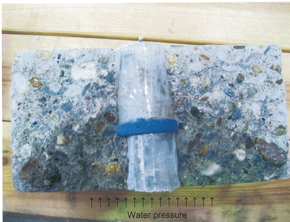
Fig. A4: Sample 3: fibrous-concrete pipe ( \varnothing_{\text{inside}} = 22 \text{ mm} , \varnothing_{\text{outside}} = 40 \text{ mm} ) with sealing ring and 1 plug (negative water pressure acting on the plug)
