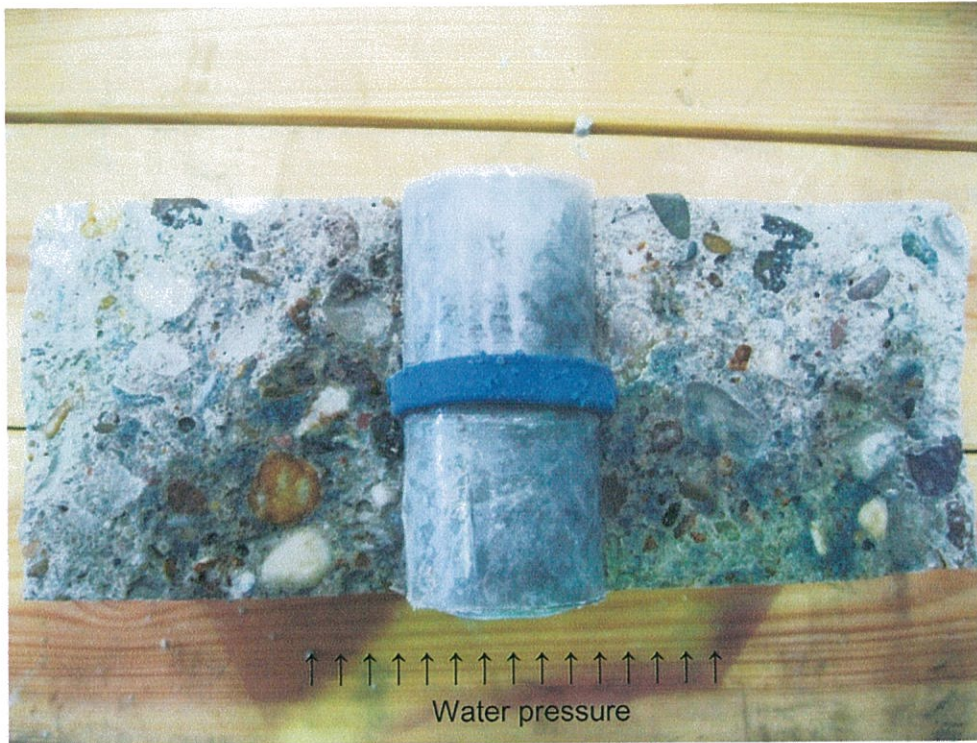
Fig. A2: Sample 1: fibrous-concrete pipe ( \varnothing_{\text{inside}} = 22 \text{ mm} , \varnothing_{\text{outside}} = 40 \text{ mm} ) with sealing ring and 2 plugs
