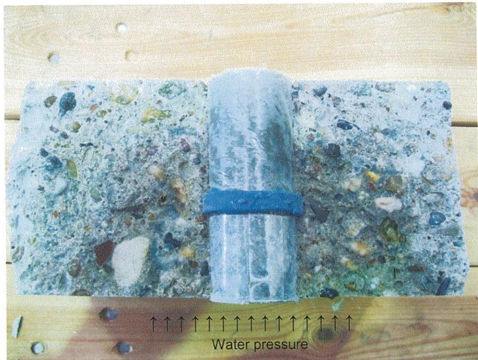
Fig. A3: Sample 2: fibrous-concrete pipe ( \varnothing_{\text{inside}} = 22 \text{ mm} , \varnothing_{\text{outside}} = 40 \text{ mm} ) with sealing ring and 1 plug (negative water pressure acting on the plug)
